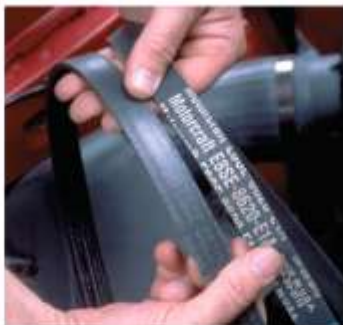
7 Match the old belt up for size with the new replacement belt.
