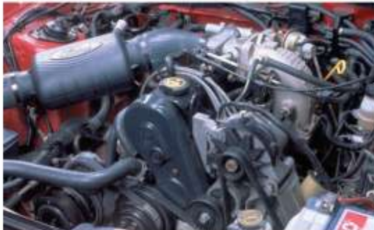
15 Start the engine and check the belt for proper operation.
