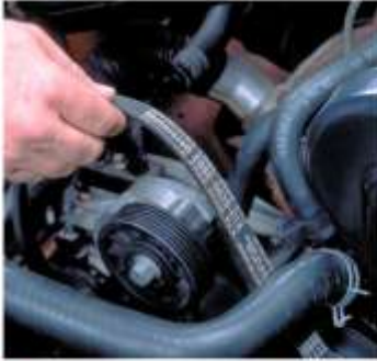
9 Install the new belt over each of the drive pulleys. Often the manufacturer recommends a sequence for feeding the belt around the pulleys.
