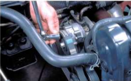
14 Tighten the tensioner or generator pulley fastener.
