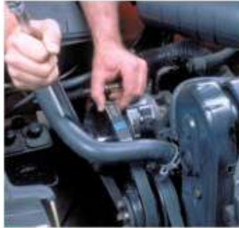
10 Pry out the tensioner or generator pulley to put tension on the belt.
