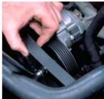
6 Pry the tensioner or generator pulley inward to release the belt tension and remove the belt.
