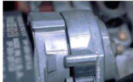
13 Pry the tensioner or generator pulley to adjust the belt to specifications.
