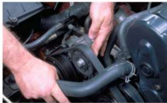
4 To replace a worn belt, locate the tensioner or generator pulley.
