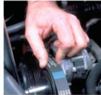
11 Install the belt squarely in the grooves of each pulley.
