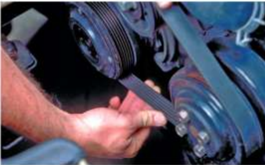
12 Measure the belt deflection in its longest span. If a belt tension gauge is available, use it and compare the tension to specifications.
