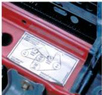
8 Observe the belt routing diagram in the engine compartment.
