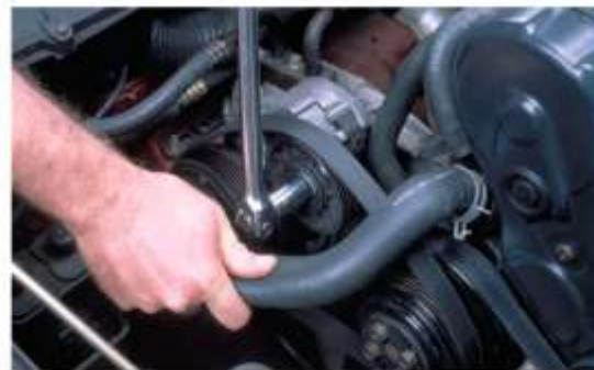
5 Loosen the hold-down fastener for the tensioner or generator pulley.
