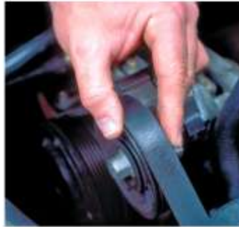
2 Look for signs of glazing.
