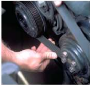
1 Inspect the belt by looking at both sides.
